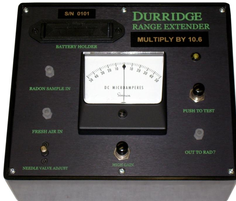
The needle valve is placed on the high radon side of the air flow path because that side has the longer capillary tubing and a slower flow rate. The pressure drop across the inlet filter on the high radon side will therefore be less than the pressure drop across the inlet filter on the fresh-air side. The needle valve is used to provide some additional pressure drop on the high radon side to bring the inlet pressure at the capillary tubing entrance to the same pressure as on the fresh-air side.
